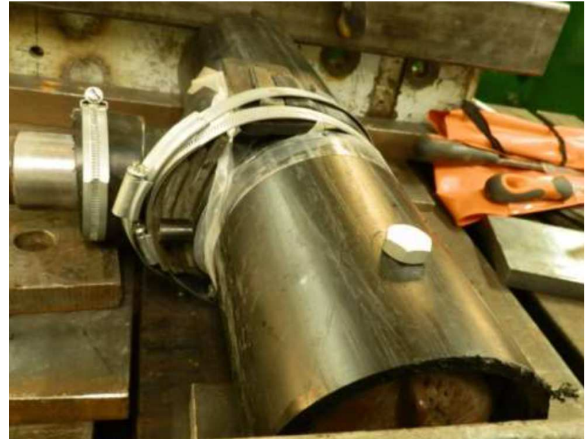
Defective Saddle connection - Pressure test
