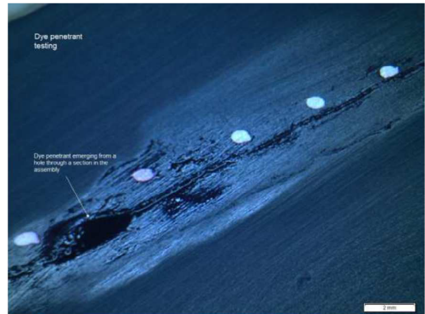
Plate 12 – Shows dye penetrant emerging from the void in the longitudinal axis
