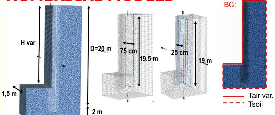
Pipes diameter = 25 mm Pipes thickness = 2.3 mm Initial temperature = 12 ° C Inlet temperature = 20 ° C
